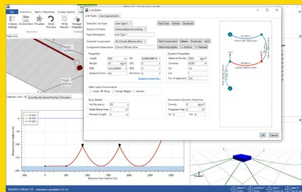
Component Properties & Intermediate Grounding
